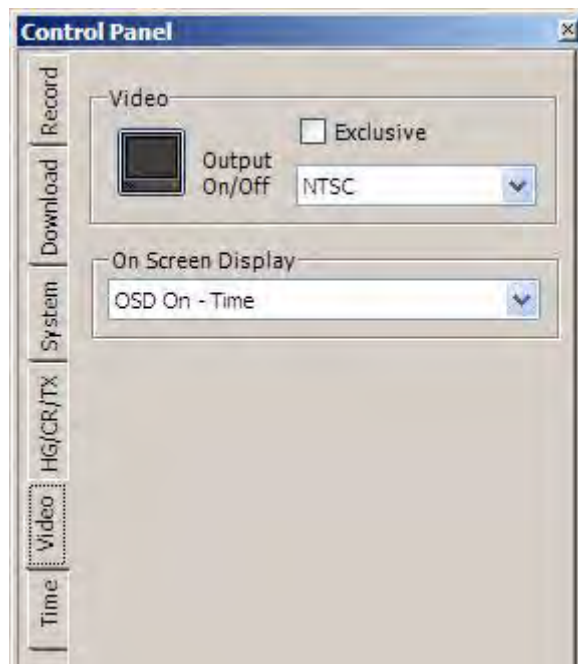
Figure 12.2: Video tab for NTSC/PAL output
