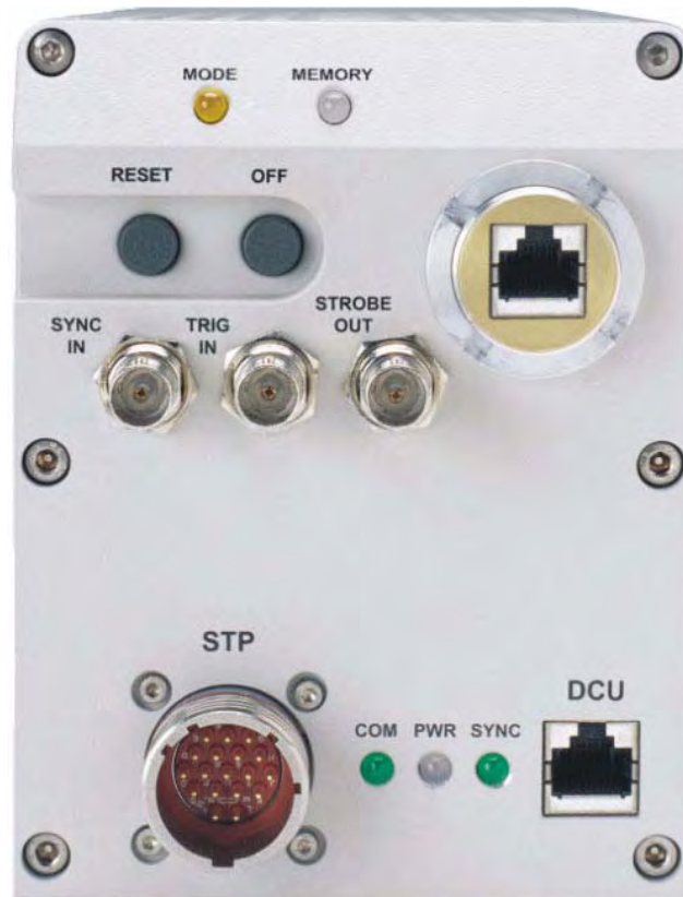
Figure 5.1: HG-100K/LE back panel
