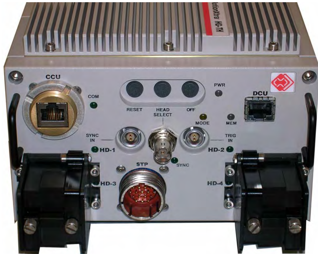
Figure 5.6: HG-TH Camera Controller
